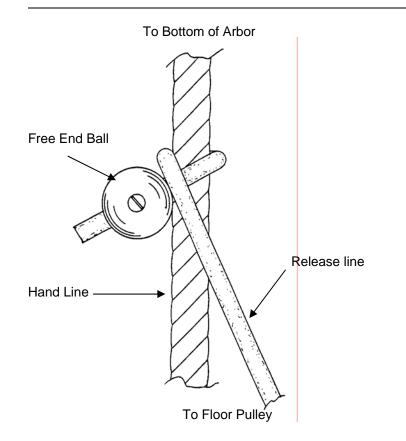
This type of system requires some practice and angle at which the release line is attached to the handline is critical. Too little of an angle, and the curtain will not deploy. Too much of angle and the release line won't hold. Additional weight may be added to the release line either before of after the floor block to aid in the quick freeing of the line. If you are having difficulty with setting your release, contact a professional stage rigging company.
