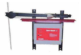
To ensure proper operation, the tension in the release line must be set between 5 & 40 pounds (3 & 18 Kg). See the fire safety curtain system drawings for additional details on installing the release line and rigging for your specific system.
